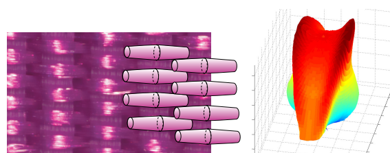
Figure 12: Left: Purple satin macro photograph with sketched double cones. Right: deduced microfacet distribution (log plot).
