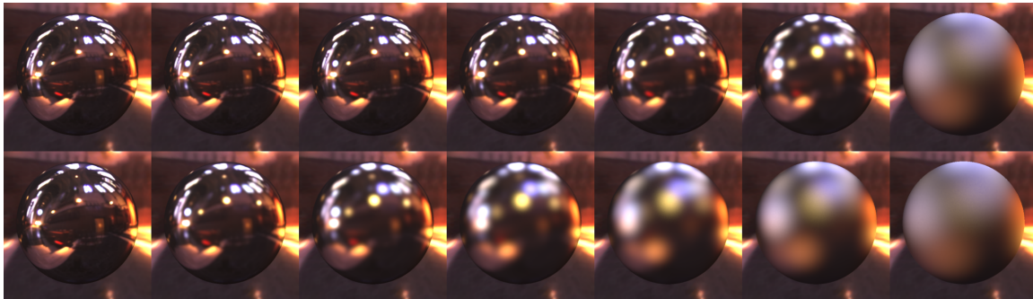
Figure 6-2: The Ward model, varying along the roughness dimension ( \alpha = 0.01 to 0.37 ). Row 1: uniformly spaced according to the BRDF space L^2 metric, Row 2: uniformly spaced according to our image metric.
