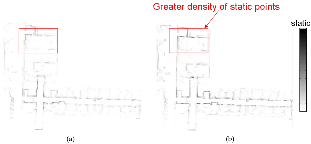
Figure 6-23: Static histograms of DPG-SLAM (on the left) and DPG-SLAM-NR (on the right) active maps from 60 passes through the University of Tübingen Robot Lab. The density of static map points is shown as being darker in the images.
