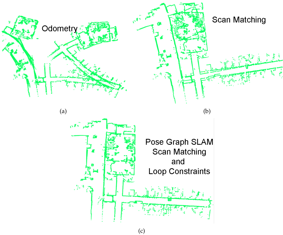
Figure 3-7: Example maps generated from pure odometry, scan matching, and pose graph SLAM using iSAM (incremental smoothing and mapping) [36].
