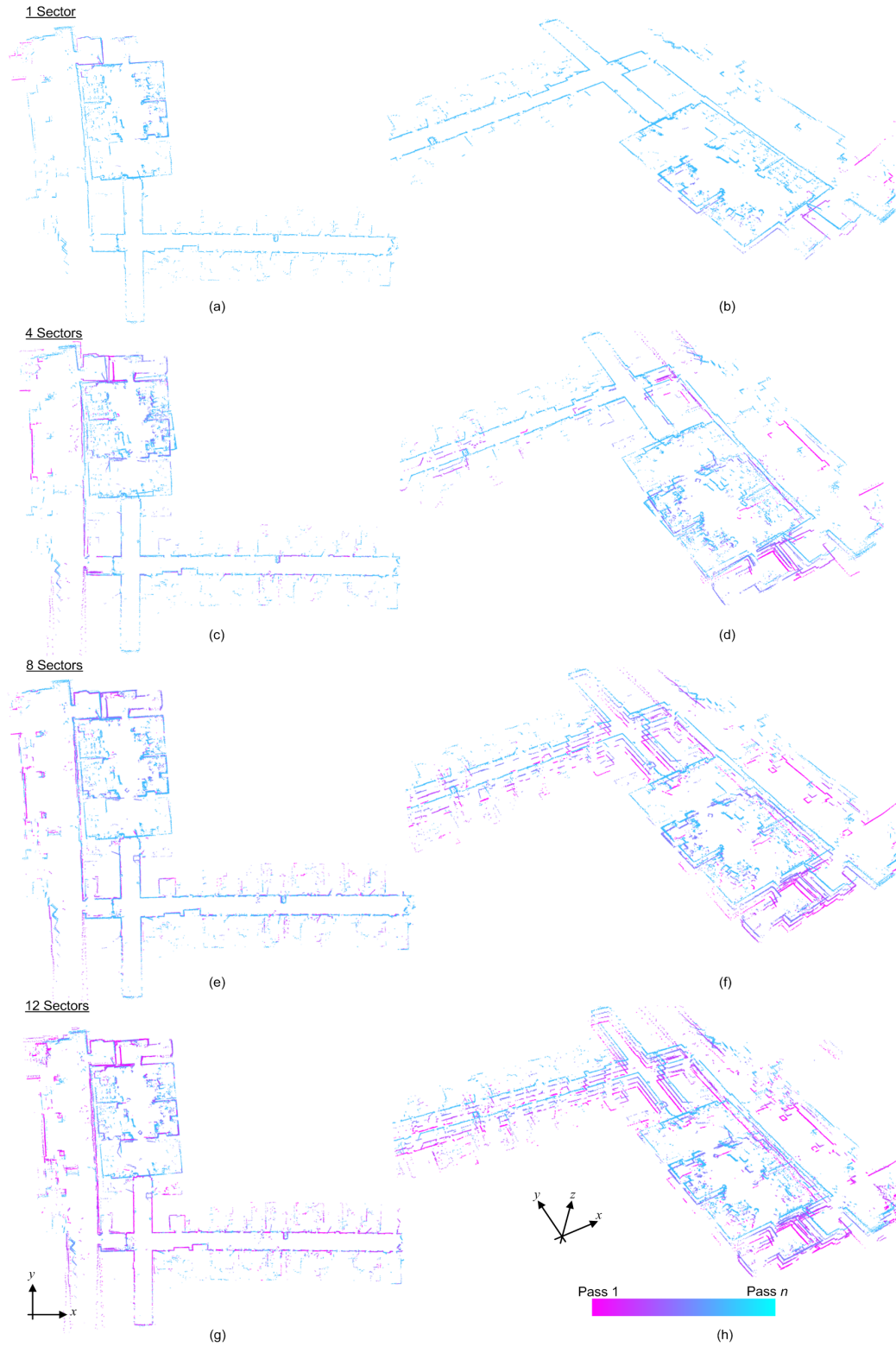
Figure 6-30: The active maps generated after applying DPG-SLAM where nodes and edges are removed.
