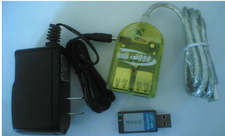
Figure 5-7: A beacon in the current version of our system consists of a USB hub (top right), AC adapter (left), and USB Bluetooth adapter (bottom right).
