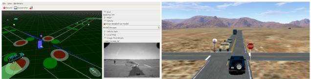
Fig. 2. (a) Screenshot of the real-time visualization tool running "live" for an intersection testing scenario, showing RNDF and vehicle navigation information (white, green, red), lidar (blue, yellow) and camera (lower right) data, and vehicle tracker output (blue solid in intersection). (b) Screenshot of SimCreator simulation environment, including MIT vehicle and traffic vehicles.
