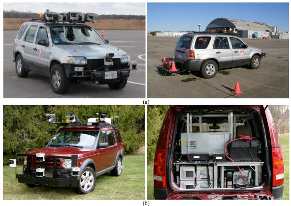
Fig. 3. Team MIT's two autonomous vehicles. (a) Talos I, a Ford Escape. (b) Talos II, a Land Rover LR3.
