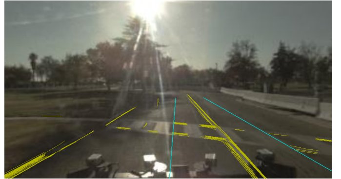
Fig. 1. Our system uses many asynchronous heterogeneous sensor streams to detect road paint and road edges (yellow) and estimate the centerlines of multiple travel lanes (cyan).
