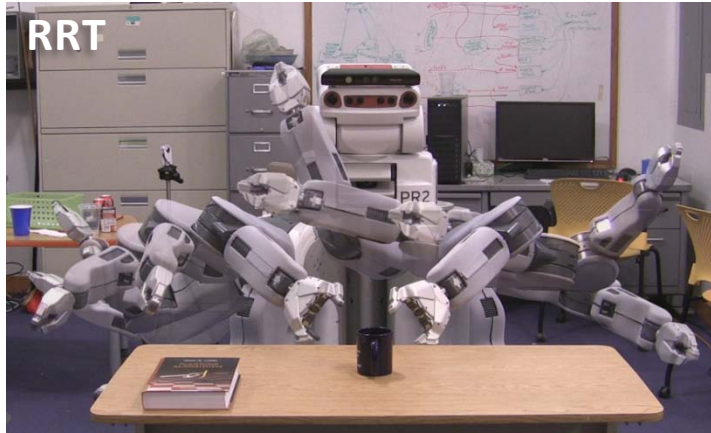
Time-lapse images of RRT and BT+RRT* trajectories after 2,000 iterations (12DOF)
