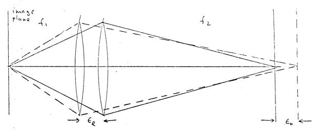
$$d = f_1 + f_2 = \frac{f_1^2}{f_1 - f_2}; :: f_1 = \frac{d - \int d^2 + df_2}{2} = f \left[ \left( \frac{d - 2f_1^2}{2f_1^2} \right)^2 + 1 - \int \left( \frac{d - 2f_1^2}{2f_1^2} \right)^2 - 1 \right]$$
