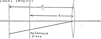
The transformation of coordinates simply multiplies distances from the optical axis by  $f_1/f$ . This introduces two new effects:
