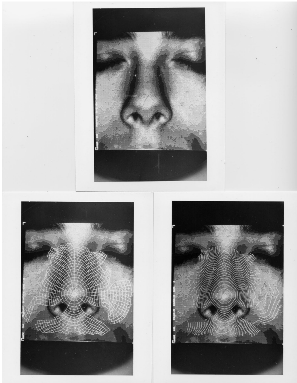
Figure 1. Recovery of shape from shading using the characteristic strip expansion method. A. Gray-level image. B. Base characteristics superimposed on the gray-level image. C. Contour map constructed from the three-dimensional characteristic strips.
