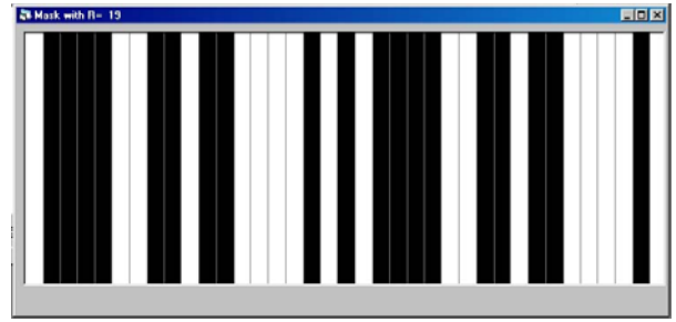
Fig. 10. One-dimensional mask pattern used in moving gamma ray detector array, based on quadratic residues for p = 19 .
