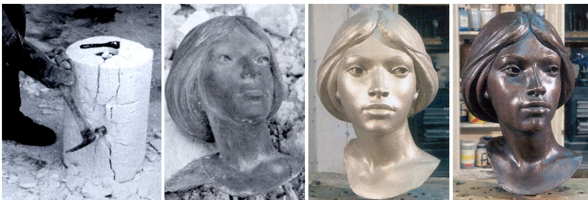
Figure 10.7: These photographs of the lost wax casting process from Langland [1999] follow the process after the stages illustrated in Figure 10.6. The outer layer of clay is broken away with a hammer to reveal the sculpture. After polishing and sandblasting, the raw metal is bright and shiny. Different chemicals are applied to the sculpture to achieve a particular patina and the model is sealed with a coat of wax.
