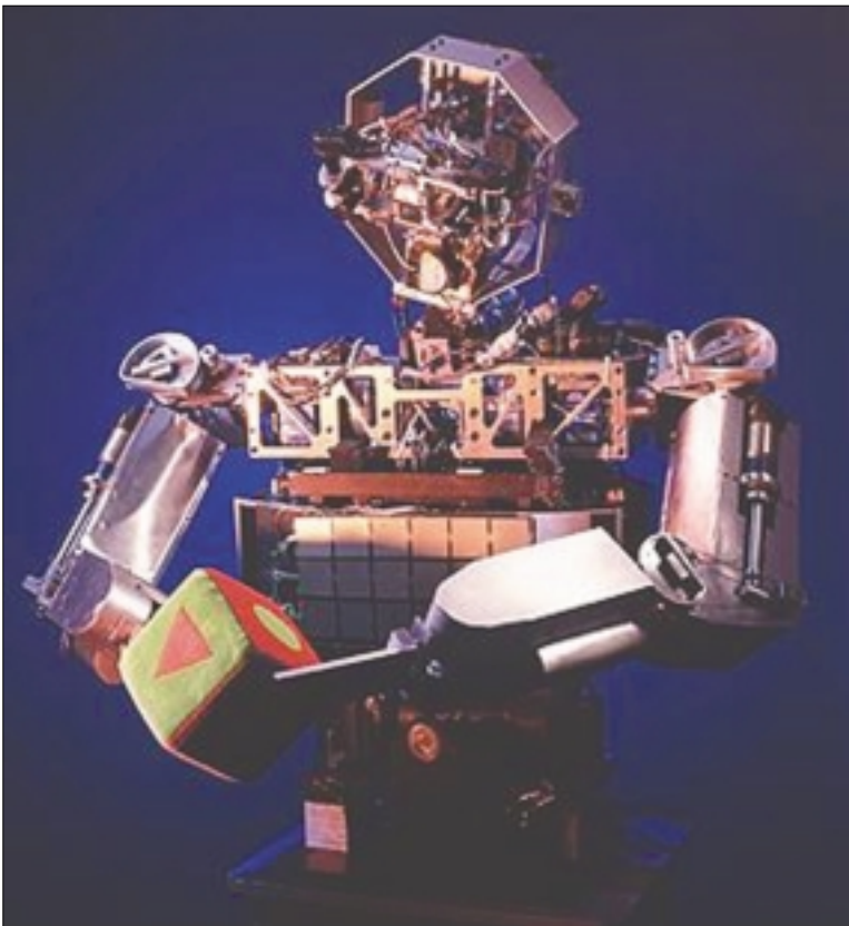
Figure 1. Our upper-torso development platform, Cog, has 22 degrees of freedom that we specifically designed to emulate human movement as closely as possible.
