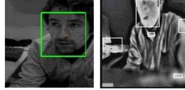
Figure 7: (Left) Face detected and window used for recognition. (Right) Heat detection from the thermal camera image.
