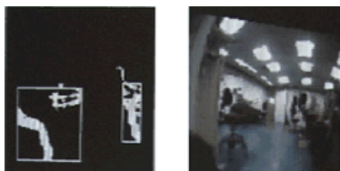
Figure 8: (left) Blobs of strong edges detected from (right) a rectified image
