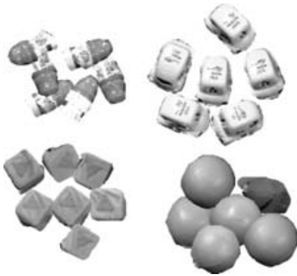
Figure 12 Once objects have been segmented from the background, they are much easier to distinguish from each other since the irrelevant similarity of their shared environment is eliminated. To build object models, the robot clusters all the segmented views it receives based on similarity of their color histogram. This figure shows samples from four of the clusters found, corresponding to the four objects used in Section 7. Note the baseball cap classified with the ball, lower right—a young child wandered by the robot while we were collecting data and got it to poke his cap.
