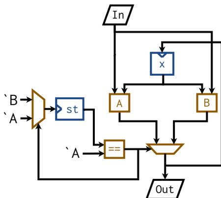
In this simple example, the circuits generated for  $st$  and  $x$  are both Muxes of the values computed by each rule, predicated by the
