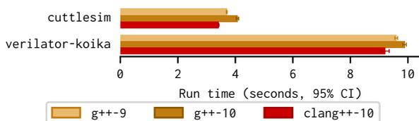
**Figure 3: Performance of Verilator and Cuttlesim models**
