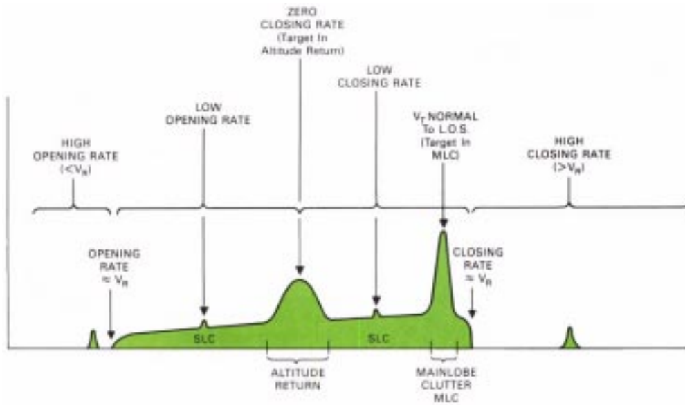
Figure 2.14 Clutter Spectrum for a Forward-Looking Radar [Stimson, 1998]
