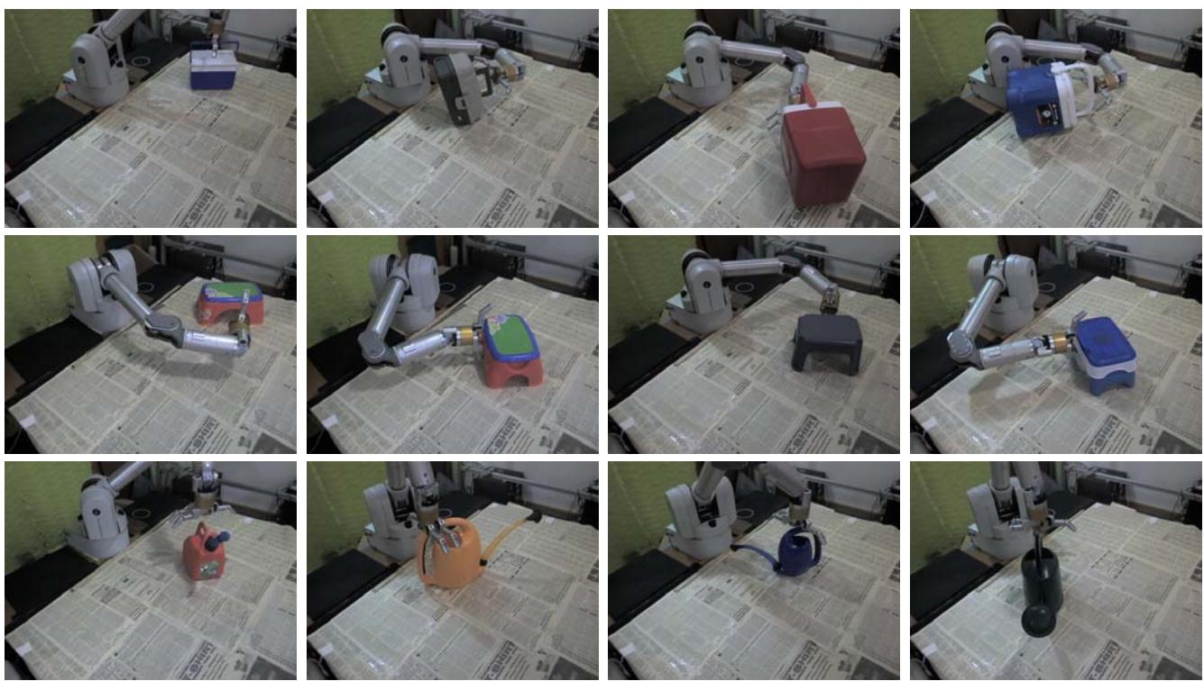
Fig. 10. Four grasps for each of the three classes (from top to bottom: coolers, stools, and watering cans).
