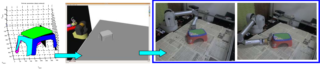
Fig. 7. From left to right: The estimated 3D instance is imported into the OpenRave [5] system and used to select a grasp from a pre-stored table that is kinematically feasible.
