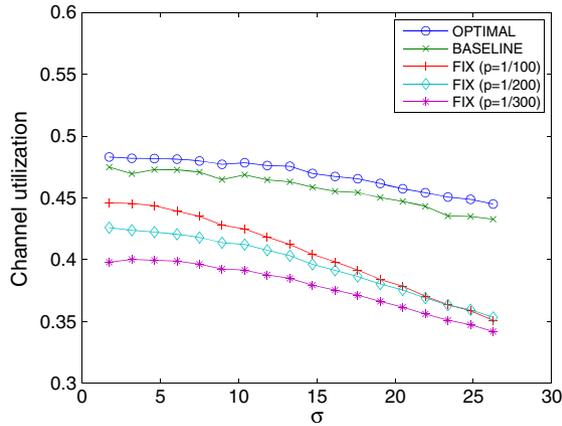
Figure 7. Comparison of channel utilization under different  $\sigma$ 's.
