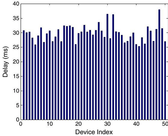
Figure 14. Average delays of individual machines for  $M = 50$ .
