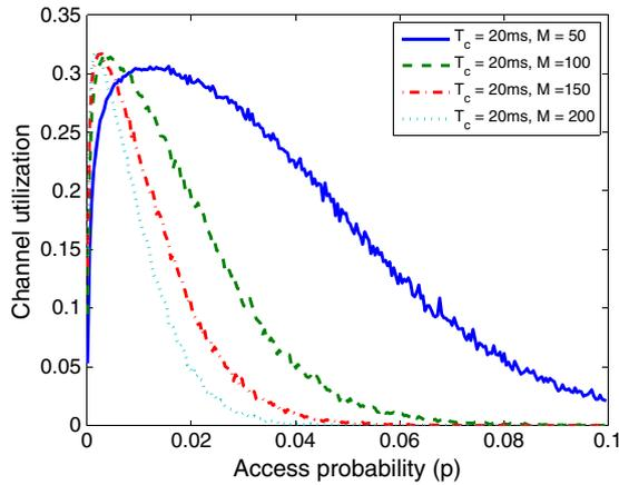
Figure 3. Channel utilization versus  $p$ :  $T_{total} = 100$  ms and  $T_n = 20$  ms.
