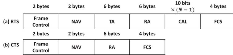
Figure 11. (a) Request-to-Send and (b) Clear-to-Send frames.
