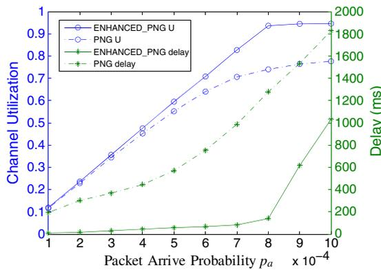
Figure 15. Comparison of channel utilization and delay under different  $p_a$ 's.
