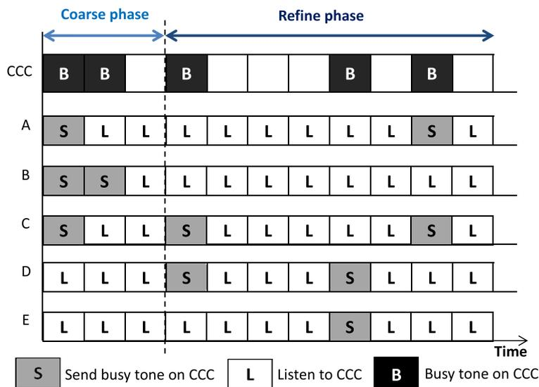
Figure 4. An example of the proposed estimation algorithm:  $M = 5$ .
