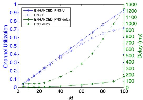
Figure 13. Comparison of channel utilization and delay under different  $M$ ’s.
