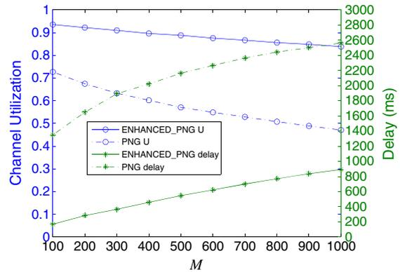
Figure 16. Channel utilization and delay in large scale networks.
