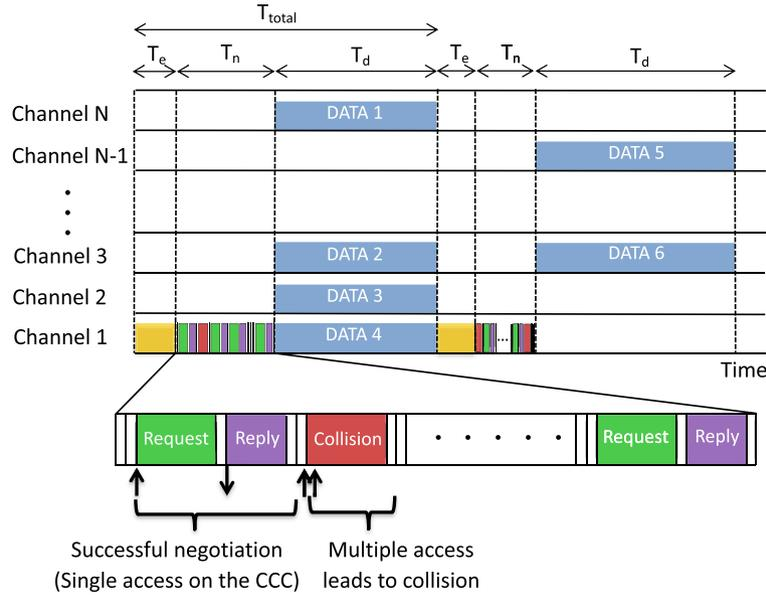
Figure 1. Timing structure of the proposed protocol.
