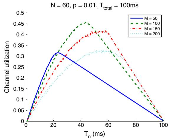
Figure 2. Channel utilization versus  $T_n$ :  $T_{total} = 100$  ms and  $p = 0.01$ .
