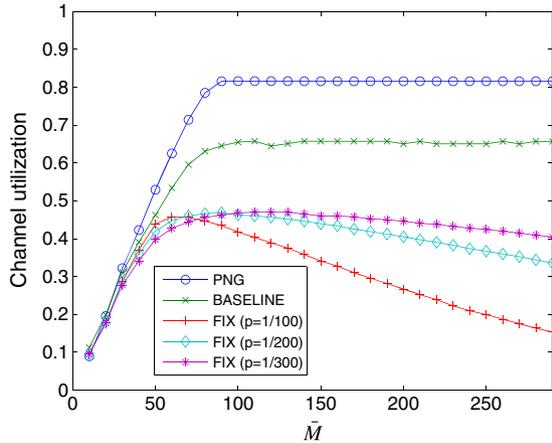
Figure 9. Comparison of channel utilization: with versus without pair-and-go.
