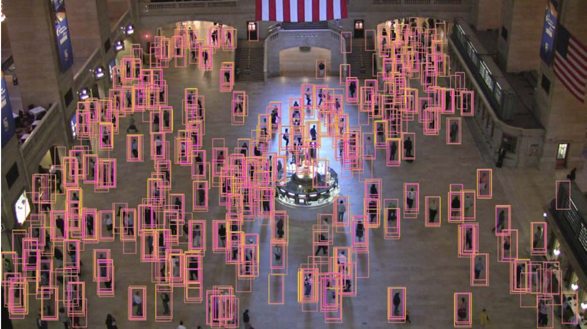
Figure 3-22: Multiple Detections : The magenta and yellow bounding boxes indicate every positive detection made by the INRIA-new + hard + GrandCentral classifier in this image. Note that for nearly every actual pedestrian, there are many positive detections.
