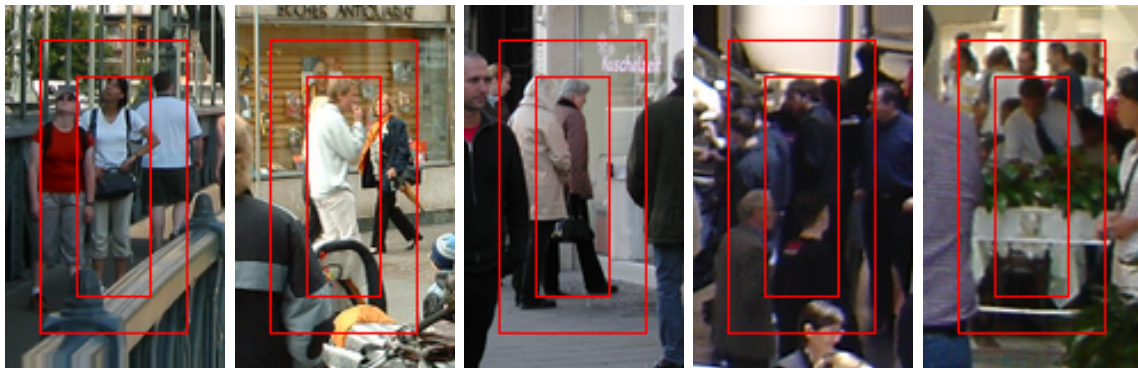
Figure 3-17: Positive Training Images from the INRIA-new Dataset : These images are people that were excluded from the INRIA-orig dataset. The outer red box shows the detector window boundary. The inner red box shows the canonical pedestrian size within a window.
