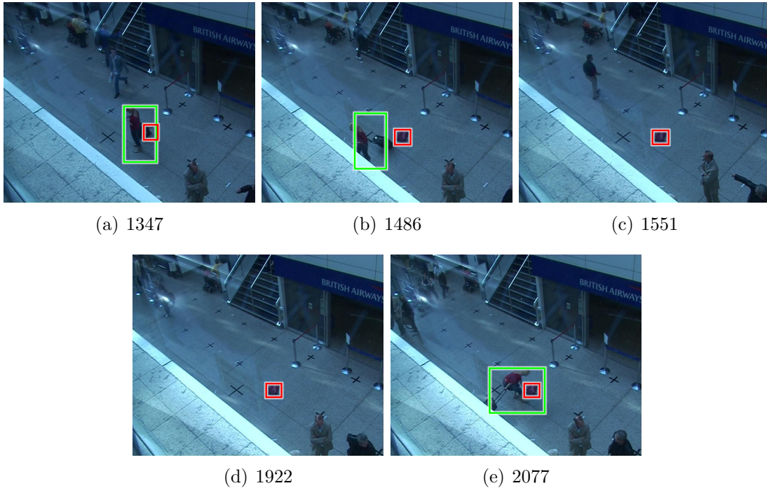
Figure 6-10: S07 Key Frames : We detect the loiterer (green bounding boxes), the fact that she drops and abandons a purse (red boxes), and that she is the person who later returns to pick up the purse.
