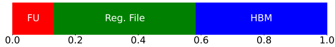
Fig. 5: Power breakdown for NoCap across FUs, reg. file, and memory (HBM) for a 16M-constraint statement.
