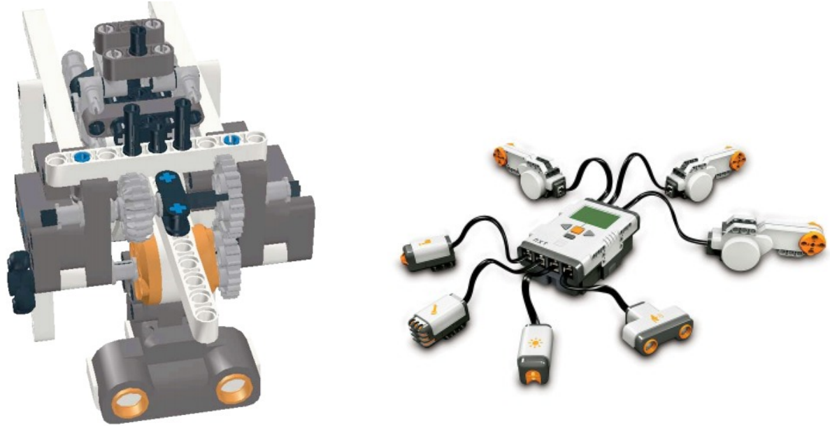
Fig. 2. Left: Example of our robot arm. Right: Lego Mindstorms set with his 3 motors and 4 sensors.
