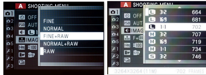
FIG. 11 Fujifilm image quality menu (left) and image size menu (right).
