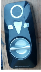
Figure 1: View of one smart lock (Okidokeys) from the interior of the home. All locks augment or replace the interior deadbolt’s turn knob with the smart lock’s electronically controllable component; however, all locks can be manually operated from the inside and they maintain a traditional keyhole on the exterior of the door.
