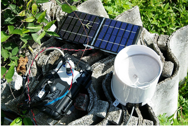
Figure 8. Precipitation Sensor Node Consisting of Electronics, Sensor and Photovoltaic Board
