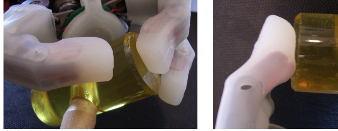
Figure 4-10: In Domo's hands, passive compliance of varying stiffness is integrated into the actuator, finger tip, and silicone skin. Although difficult to model, a compliant skin allows the robot to expand the contact surface during grasping, greatly improving grasp stability.
