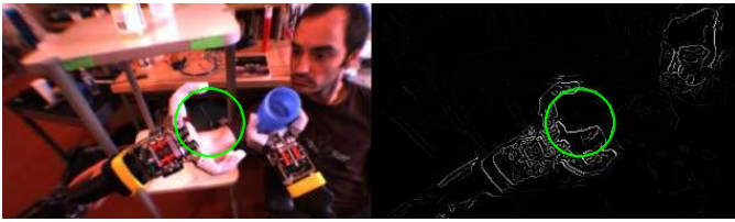
Fig. 4. The robot’s view as it transfers an object to its right hand to its left. The everyday environment includes the shelf, a person, as well as natural lighting and a cluttered background. The edge motion (right) of the hand is used to estimate the location of the contact surface (green). This estimate is then used to visually servo the contact surface in the scene. In addition, the robot actively adapts its posture such that it can more easily view the controlled features.
