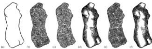
Figure 8: Direction fields on the Venus. (a) Silhouettes alone do not convey the interior shape of the surface. (b) Raw principle curvature directions produce an overly-complex hatching pattern. (c) Smooth cross field produced by optimization. Reliable principal curvature directions are left unchanged. Optimization is motivated by the principal curvatures. (d) Hatching with the smooth cross field. (e) Very smooth cross field produced by optimizing all directions. (f) Hatching from the very smooth field.
