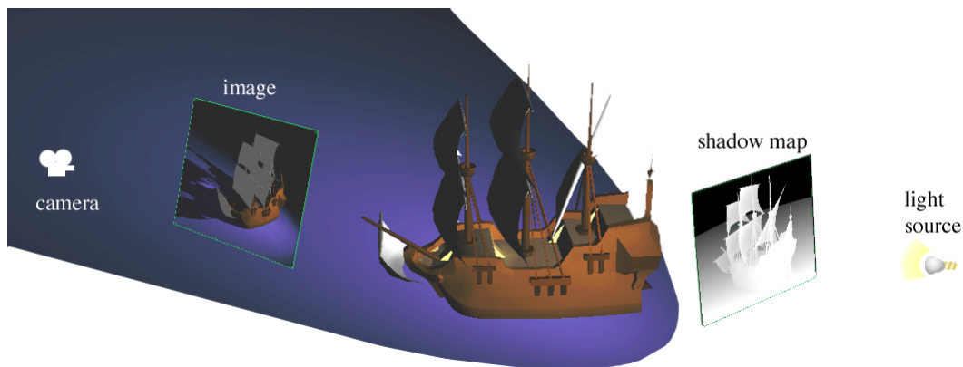
Figure 11.1: Shadow map principle. A shadow map is computed from the point of view of the light source (z-values are represented as grey levels). Then each point in the final image is tested for shadow occlusion by projecting it back in the shadow map (gallion model courtesy of Viewpoint Datalab).
