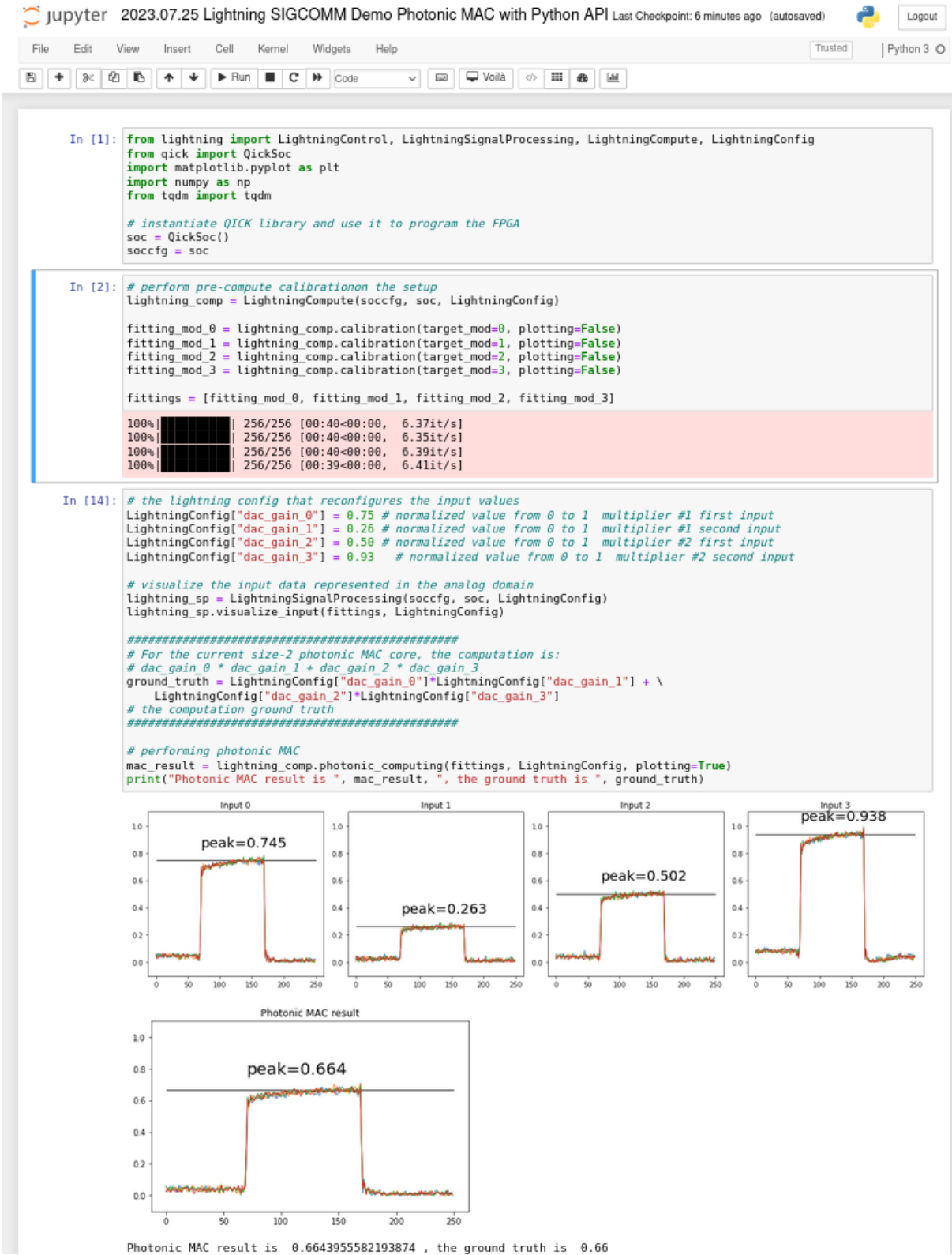
Figure 27: Benchmarking photonic vector dot product on LIGHTNING's prototype with our Python API.
