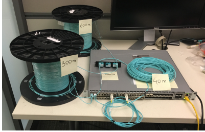
Figure 10: Our 10G-SR testbed. We stitch short fibers together with fiber connectors to emulate long fibers. We concatenate 600m, 300m, 40m fibers together to emulate a 940m fiber. Two 300m 10G-SR Finisar transceivers [8] are attached to the fiber on both ends. Switch ports are on and we can send traffic through with BER of around 10^{-8} .
