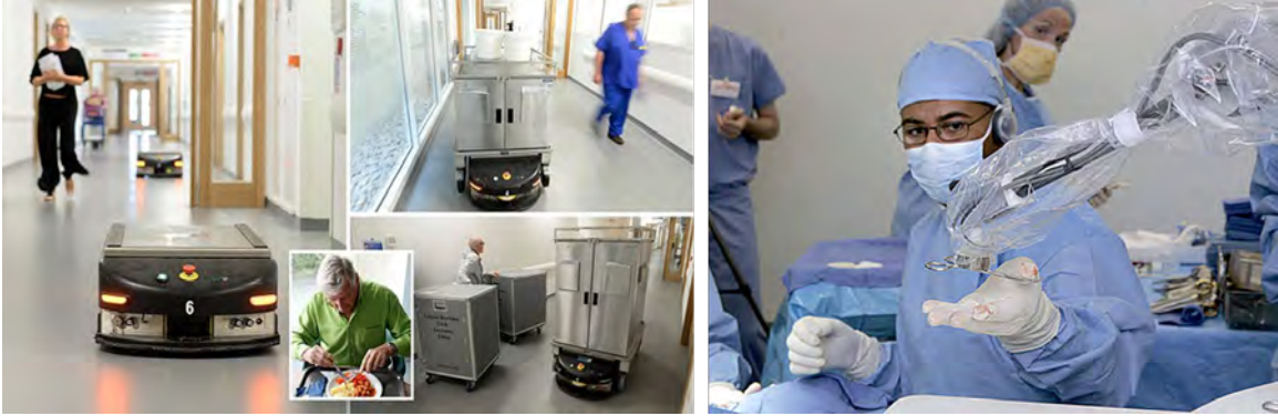
Figure 1-3: This figure depicts (left) hospital service robots transporting meals within a hospital. These robots, deployed at Southmead Hospital (Bristol, England), are the Transcar LTC 2. They are developed by Swisslog Telelift LTC, a member of KUKA Group. To the right, a surgeon is depicted working with Penelope, a robotic surgical assistant developed by Robotic Systems and Technologies, Inc. (New York, NY). Penelope must be commanded by the surgeon via voice commands. Images are credited to KUKA and Robotic Systems and Technologies, Inc., respectively.
