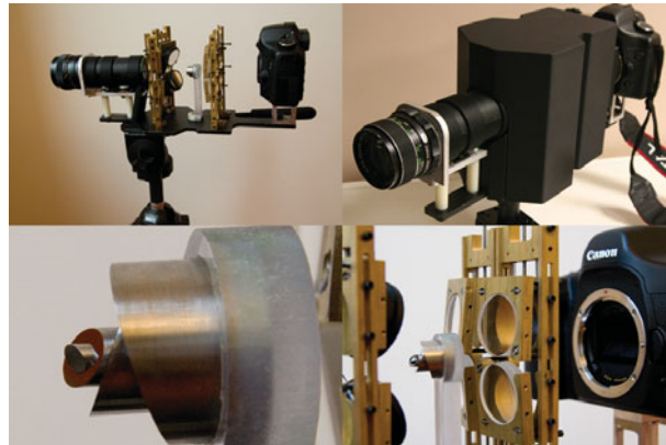
Figure 1: Photographs of our prototype optical system to capture multi-aperture images. The system is designed as an extension to a standard DSLR camera. The lower right image shows a close-up of the central mirror used to split the aperture into multiple paths.
