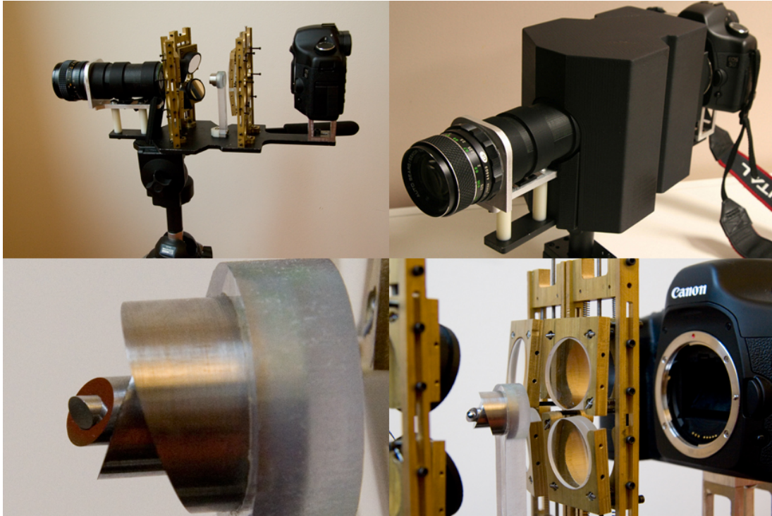
Figure 3-1: Photographs of our prototype optical system to capture multi-aperture images. The system is designed as an extension to a standard DSLR camera. The lower right image shows a close-up of the central mirror used to split the aperture into multiple paths.
