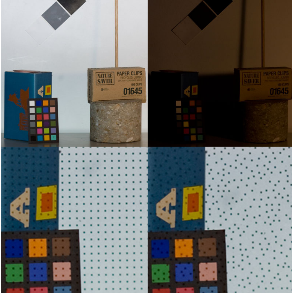
Figure 4-1: Top: A scene photographed with and without flash. Bottom: Close-ups of two possible samplings of flash and no-flash pixels using our multiplexed flash illumination.
