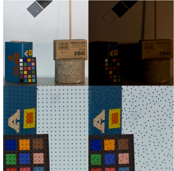
Figure 1: Top: A scene photographed with and without flash. Bottom: Close-ups of two samplings of flash and no-flash pixels using our multiplexed flash illumination.
