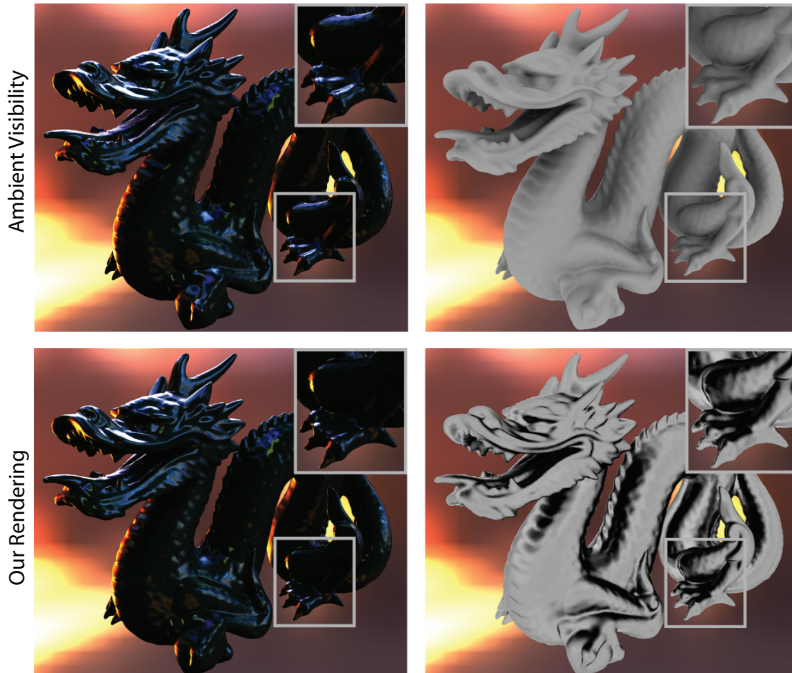
Figure 7: A Dragon model rendered with our real-time environment mapping method. Top row: visibility approximated as the percentage of the occluded hemisphere (Ambient Visibility). Bottom row: Our Spherical Harmonic visibility approximation. The left column shows full renderings and while the right column shows the visibility weights per pixel. Our approximate visibility technique eliminates highlights that occur in occluded regions (e.g. see foot and inset images) when rendered using ambient visibility.
