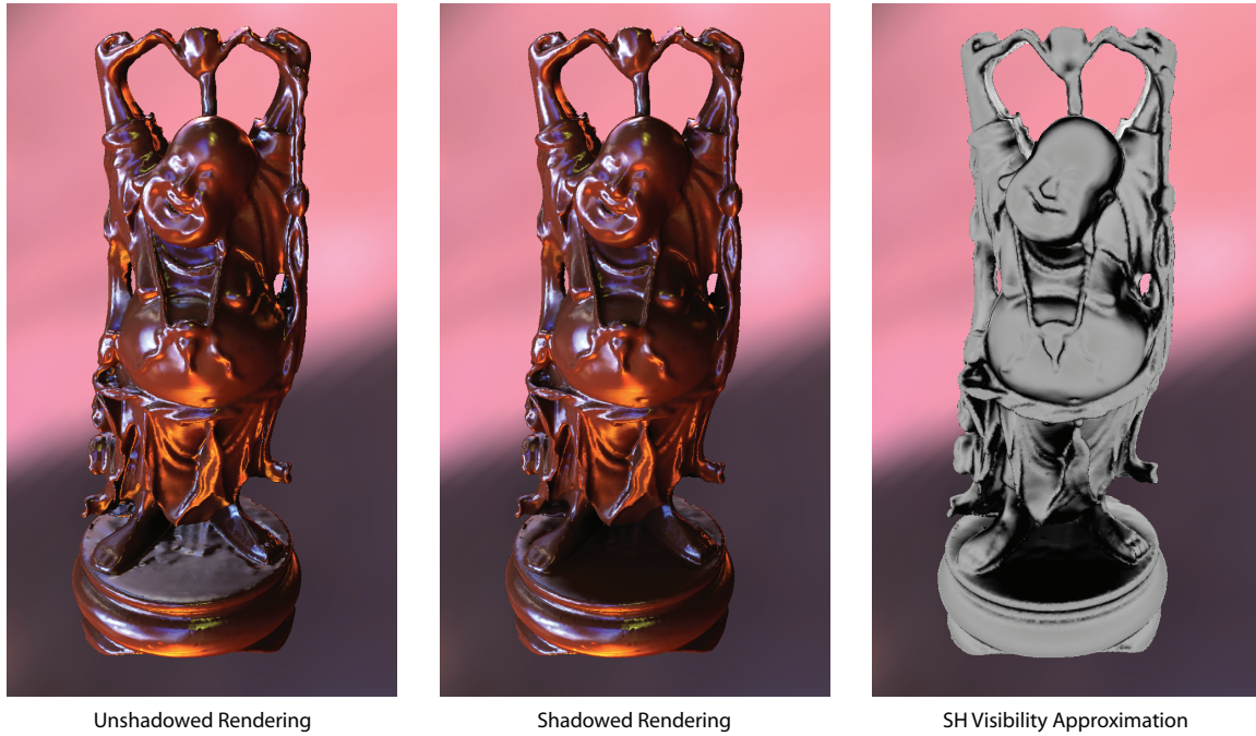
Figure 5: Visibility comparison. The same model is rendered with and without shadowing. Notice how small-scale shadow events are perceptually not important; at first glance both models look identical (upper half of model). However, larger shadows are quite noticeable. Our visibility representation exploits this observation. Model contains 100K vertices and renders at 350Hz on a NVidia 8800.
