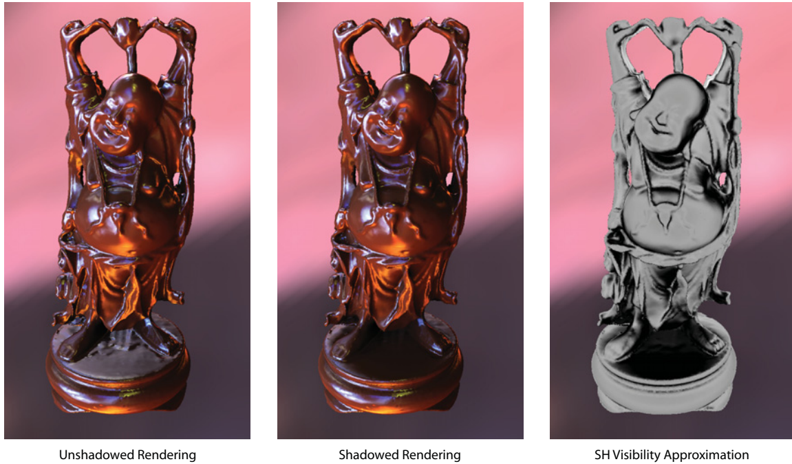
Figure 5: Visibility comparison. The same model is rendered with and without shadowing. Notice how small-scale shadow events are perceptually not important; at first glance both models look identical (upper half of model). However, larger shadows are quite noticeable. Our visibility representation exploits this observation. Model contains 100K vertices and glossy reflections render at 350Hz on a NVidia 8800.
