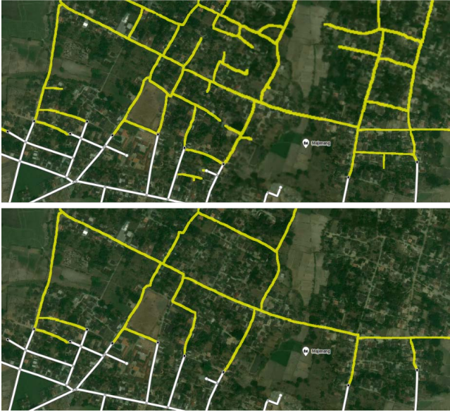
Figure 5: Pruning in MAiD. Above, the overlay includes all automatically inferred road segments. Below, pruning is applied to retain only segments corresponding to major roads.
