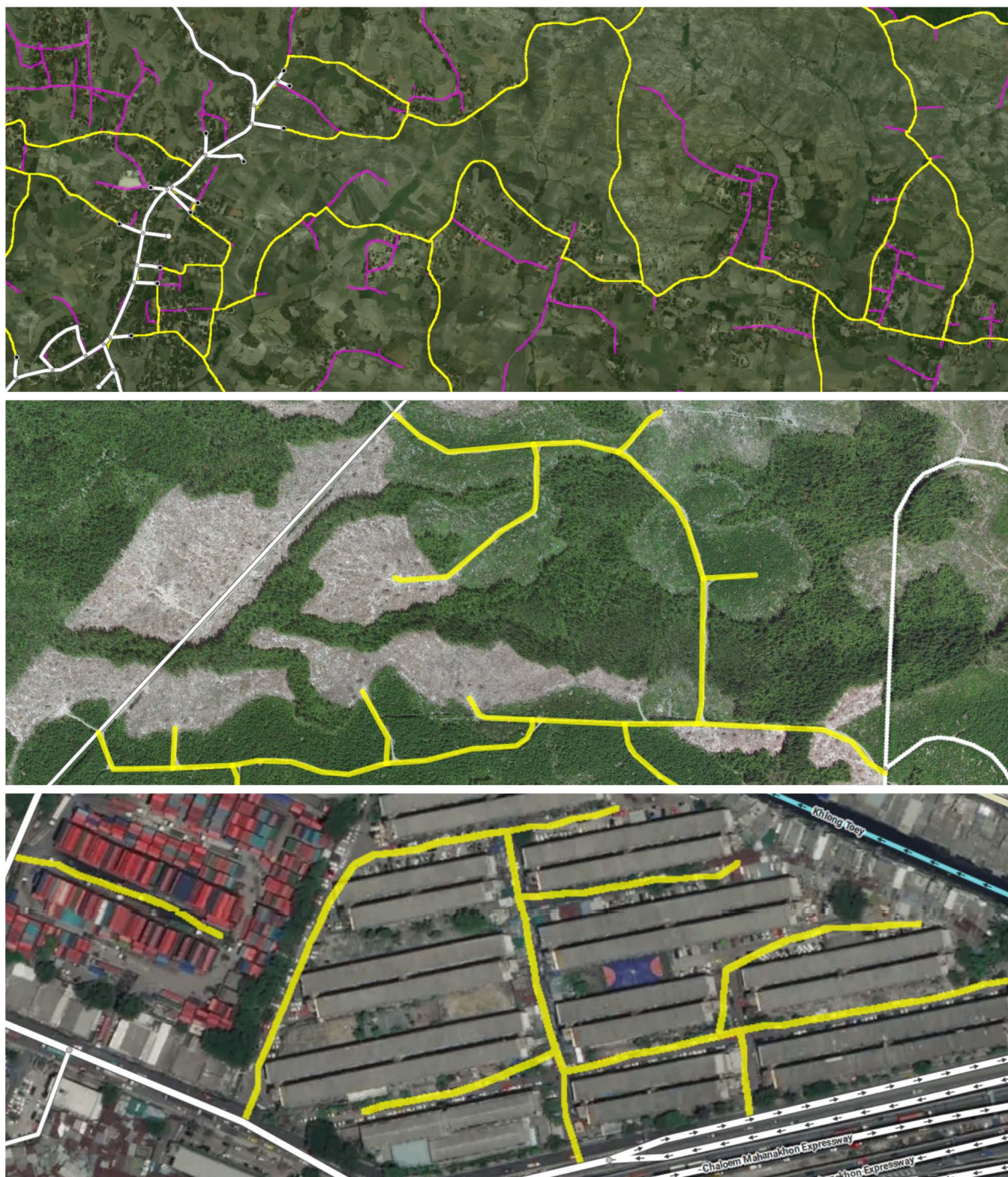
Figure 12: Qualitative results from MAiD with our map inference algorithm. Segments in the existing map are in white. We show our pruning approach applied on a region of Indonesia in the top image, with pruned roads in purple and retained roads in yellow. The middle and bottom images show connected components of inferred segments that the teleport feature pans the user to, in Washington and Bangkok respectively.
