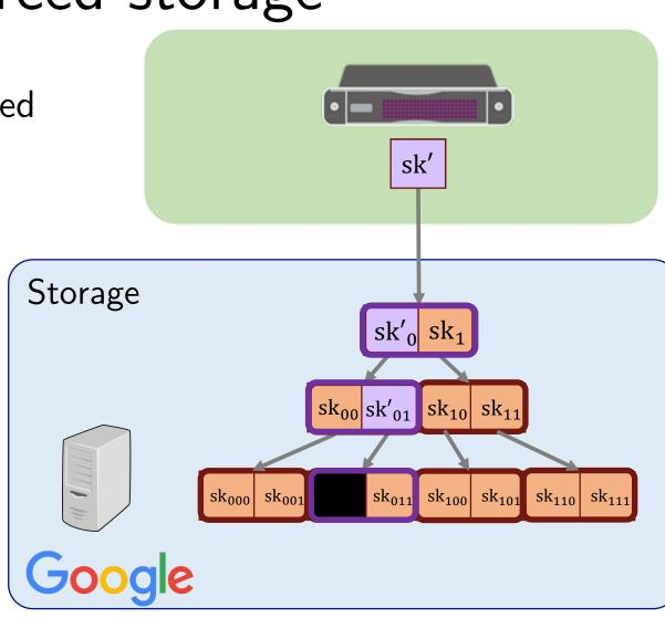
Each read/write/delete requires a number of symmetric-key crypto ops logarithmic in the array size.
