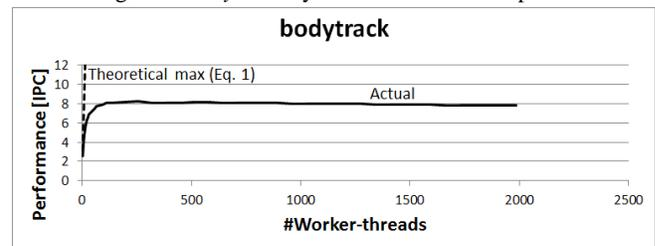
Figure 9: *bodytrack* performance – saturation at ~128 threads
