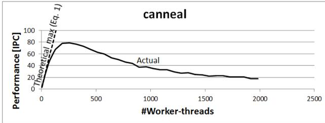
Figure 12: *canneal* performance – peak at ~256 threads
