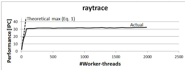
Figure 14: *raytrace* performance – saturation at ~80 threads
