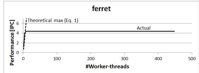
Figure 16: *ferret* performance – saturation at ~8 threads
