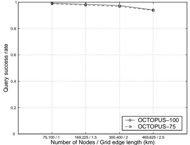
Figure 12: Octopus’s query success rates for different node densities.
