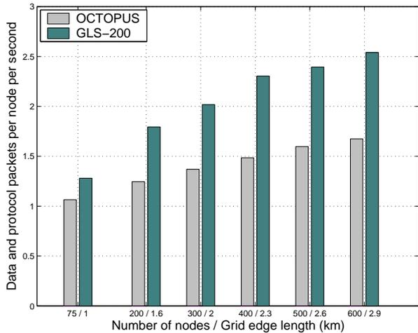
Figure 18: Octopus versus GLS: data and protocol packets sent.
