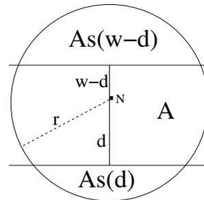
Figure 9: Node  $N$  has a forwarding hole in direction east if area  $A$  is uninhabited.
