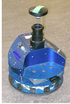
Figure 4-1: Left: The mobile robot “Samurai” used for the real world experiments, equipped with an omnidirectional camera and differential steering. Right: Mechanical specifications of the robot.
