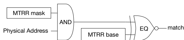
Figure 2.25: The circuit for computing whether a physical address matches a memory type range. Assuming a CPU with 48-bit physical addresses, the circuit uses 36 AND gates and a binary tree of 35 XNOR (equality test) gates. The circuit outputs 1 if the address belongs to the range. The bottom 12 address bits are ignored, because memory type ranges must be aligned to 4 KB page boundaries.
