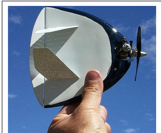
Figure 5: A micro air vehicle (MAV) built by MLB Co. [4]. This six-inch wonder toy comes with a video camera and a dispenser for cubic-centimeter sized sensor nodes. At the time of this writing, it can hit 60 m.p.h. and stay aloft for 18 minutes! Swarms of these tiny craft could rain Smart Dust upon the target area.
