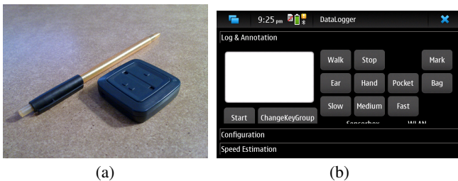
Figure 2. Nokia Sensorbox and data logging program
