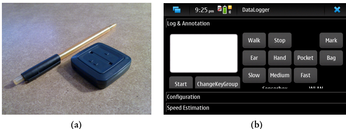
Figure 5-4: Nokia Sensorbox and data logging program
