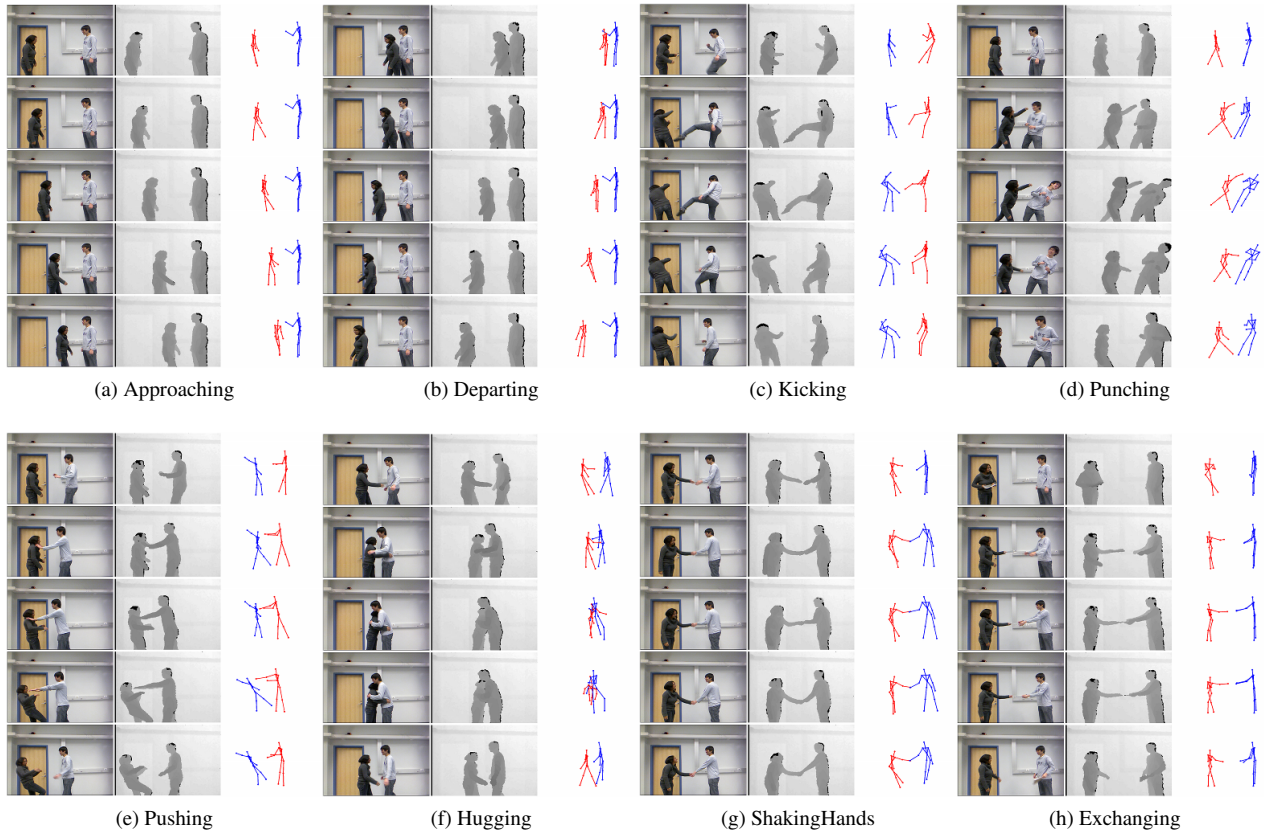
Figure 1: Visualization of our interaction dataset. Each row per interaction contains a color image, a depth map, and extracted skeletons at the first, 25%, 50%, 75%, and the last frame of the entire sequence for each interaction: approaching , departing , kicking , punching , pushing , hugging , shaking hands , and exchanging . A red skeleton indicates the person who is acting, and a blue skeleton indicates the person who is reacting.
