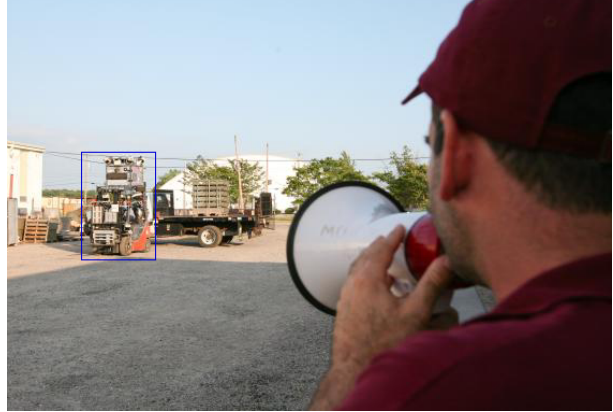
Fig. 1: Supervisor speaking through a megaphone to command a robotic forklift (in blue box) 25 meters away.
