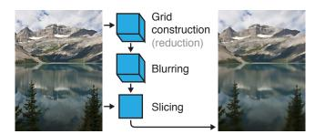
**Figure 9:** The bilateral filter smoothes detail without losing strong edges. It is useful for a variety of photographic applications including tone-mapping and local contrast enhancement. The bilateral grid computes a fast bilateral filter by scattering the input image onto a coarse three-dimensional grid using a reduction. This grid is blurred, and then sampled to produce the smoothed output.
