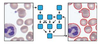
**Figure 10:** Adaptive contours segment objects from the background. Level-set approaches are useful to cope with smooth objects and when the number of elements is unknown. The algorithm iterates a series of differential operators and nonlinear functions to progressively refine the selection. The final result is a set of curves that tightly delineate the objects of interest (in red on the right).
