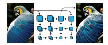
**Figure 7:** The local Laplacian filter enhances local contrast using Gaussian and Laplacian image pyramids. The pipeline mixes images at different resolutions with a complex network of dependencies. While we show three pyramid levels here, for our four megapixel test image we used eight.
