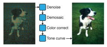
Figure 6: The basic camera post-processing pipeline is a feedforward pipeline in which each stage either considers only nearby neighbors (denoise and demosaic), or is point-wise (color correct and tone curve). The best schedule computes the entire pipeline in small tiles in order to exploit producer-consumer locality. This introduces redundant computation in the overlapping tile boundaries, but the reduction in memory bandwidth more than makes up for it.
