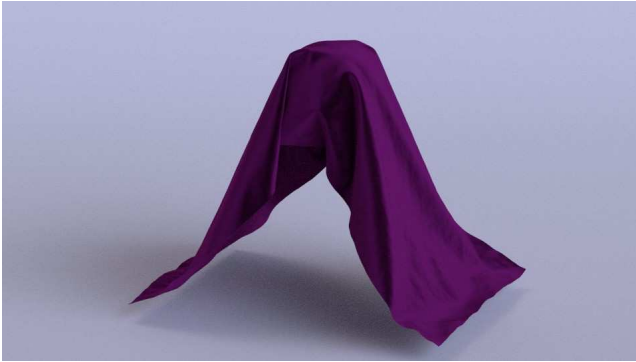
Fig. 13: Still from an Elastic Shells simulation of a cloth with 499,864 vertices, 997,012 triangle faces and 1,495,518 hinges. Elastic shells require two hyperedge sets: one for the triangle faces and one for the hinges. The Simit implementation ran at 15 frames per second on a GPU.
